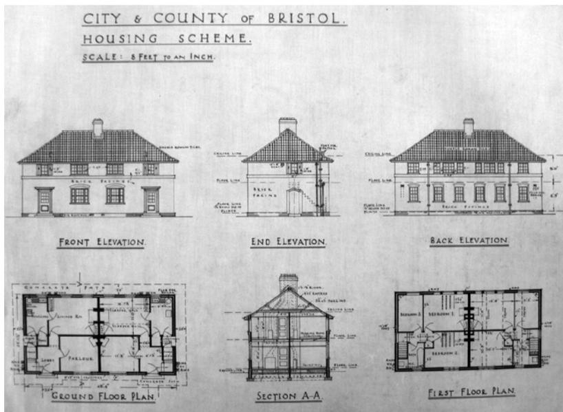
Architect's drawing of the three-bedroom WDB5 (Bristol Archives Red Label Plans 22/3/30). More than half the houses built under the Housing Act 1919 at Hillfields and Sea Mills had parlours compared with only 15 percent of those built at Southmead under the Housing Act 1924.
